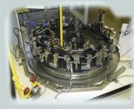
Stainless steel fixtures accommodates three bolt body lengths.
