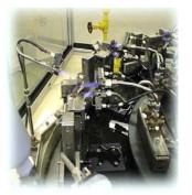
Inner and outer heat manifolds distribute filler metal throughout joint area.
