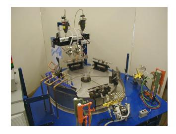
Single axis robots guide applicator guns to dispense paste filler metal to tube joints.
