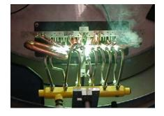
Gas/oxygen flames are gas flux enriched to minimize copper discoloration.
