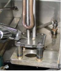
Premeasured deposits of silver-based paste filler metal are applied to joint areas.
