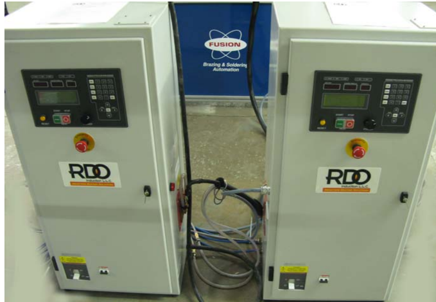
Control units for induction power supplies allow the user to monitor power output, voltage, frequency and current.
