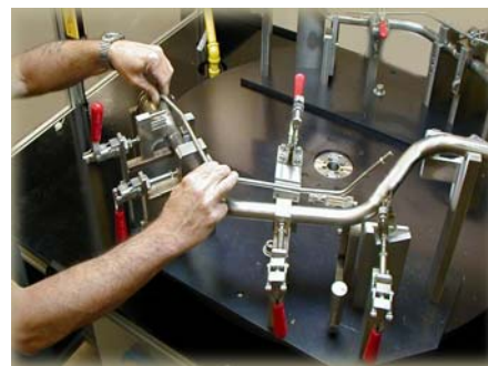
Operator positions vent tube into 27" long filler tube on locating fixture.
