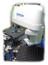
SCARA robot loads both shanks and carbide blanks into machine fixtures.
