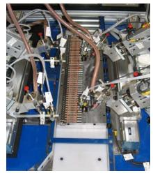
Single axis robots guide applicator guns to dispense paste filler metal to tube joints.
