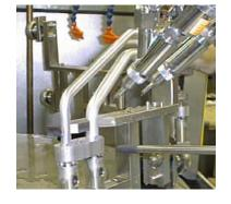
Two applicator guns dispense four deposits of paste filler metal to both joint areas.
