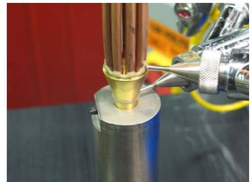
Two applicator guns dispense 360° stripes of brazing paste to all joint areas.
