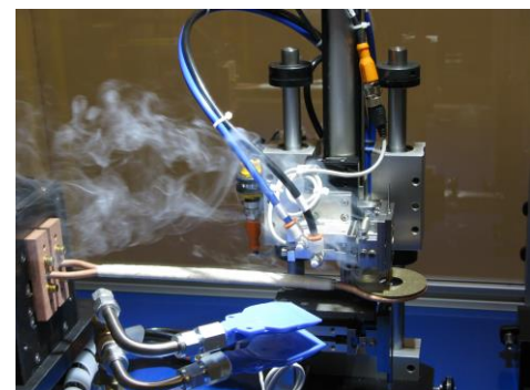
Induction workhead remelts pretinned silver brazing filler metal, completing the joint.
