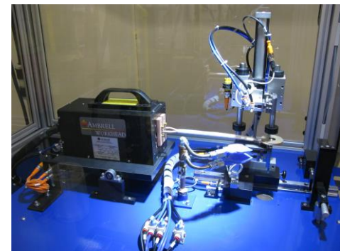
Compact brazing work station mounted within 30"x36" space.
