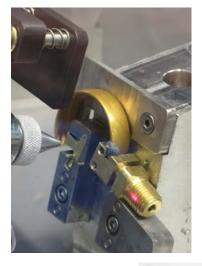
Applicator gun dispenses solder paste filler metal to joint area.
