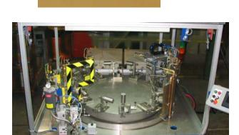
Applicator gun dispenses premeasured deposit of paste filler metal to shank.
