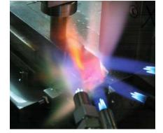
Precision, gas/oxygen burner pattern distributes filler metal throughout joint area.
