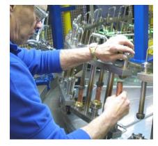
Operator loads 3 parts into each fixture.
