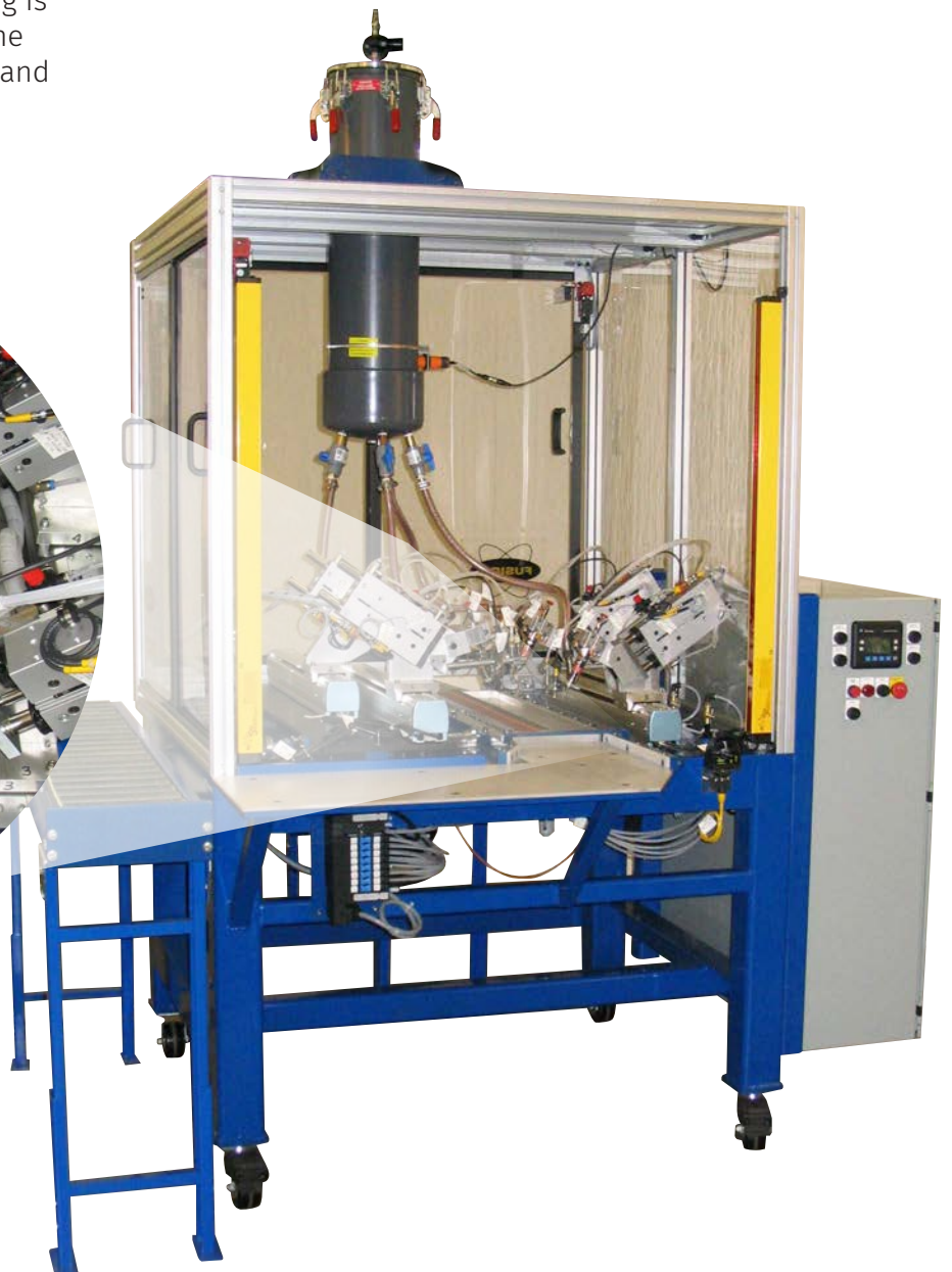
Single axis robots guide applicator guns to dispense copper paste to tube/fitting joints at 6,200 per hour. After pasting, parts are loaded into an atmosphere brazing furnace.
