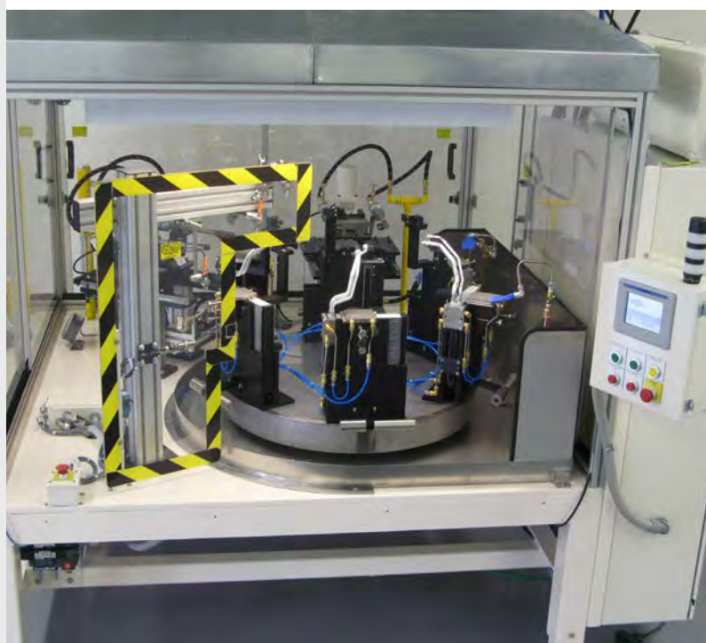
Rotary machine conveys fixtured parts through brazing/soldering alloy application, heating and cooling cycles.
